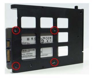
Once align, you can fasten the screws on the tray to fix the HDD. (Please make sure that the connector of the HDD is facing outward)
